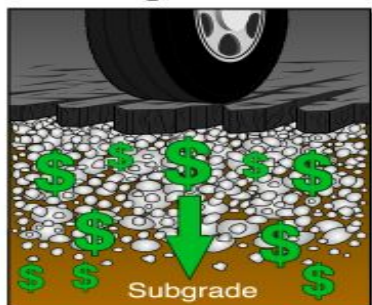
Without Geogrid Reinforcement
