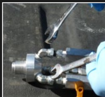
15. Tighten the manifold
