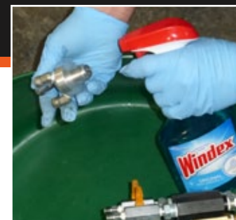
Thoroughly clean with acetone or equivalent
