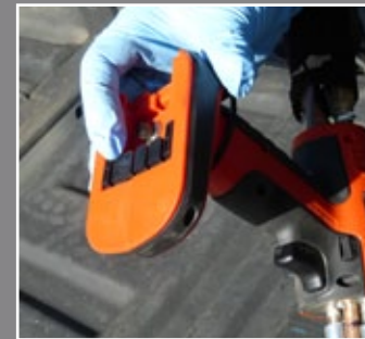
Depress button to purge air through static mixer to avoid material hardening
