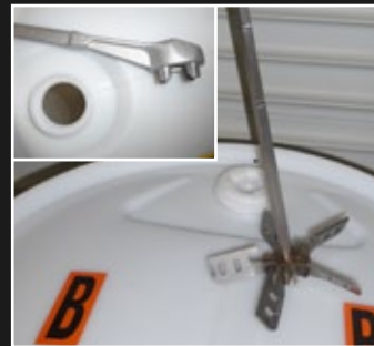
3. Pre-mix materials with fin mixer for 5 minutes
