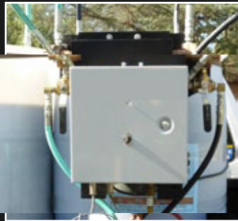
8. Move handles into upright position to recirculate material
