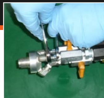
Remove the manifold from the applicator
