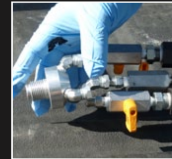
14. Attach the manifold
