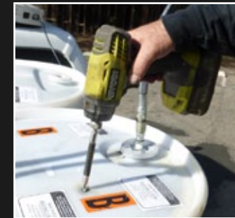
6. Vent drum with supplied vent screw
