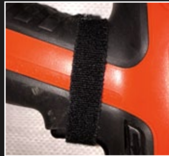
9. Use velcro strap to hold gun trigger in the on position for 5-15 minutes, depending on drum size
